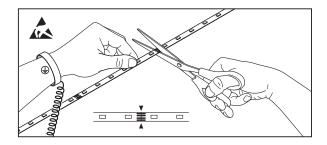
\* Connecting two segments with a soldering iron, the heating should be no more than 250 ° C and the soldering time is less than 5 seconds, please wear the electrostatic ring.
