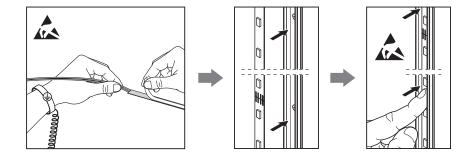
\* There are the scissors symbols on the PCB which shows you where to cut the LED strip. When cut the LED strip, please wear the electrostatic ring.
